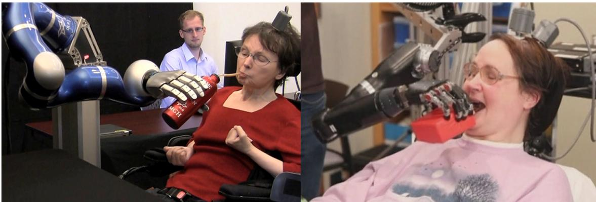
Figure 7: Real-time BMI prosthetic arm control using microelectrode arrays implanted in the motor cortex. (Left) BrainGate [34]. (Right) University of Pittsburgh [17].
